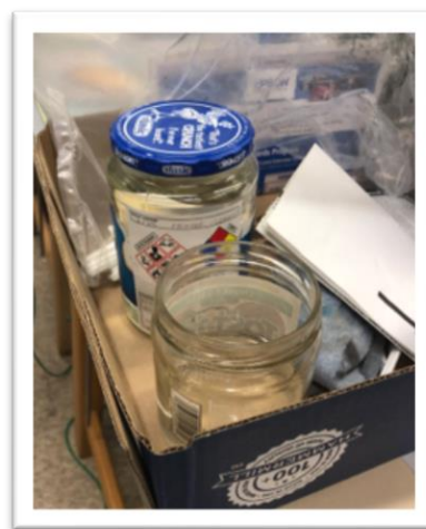
L-R: Bottles with labels that are not legible or missing, as well as chemicals being stored in food containers
